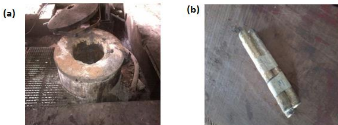
Figure-1. (a) Crucible pit furnace and (b) As-cast cylindrical rods of nickel-aluminium bronze.
