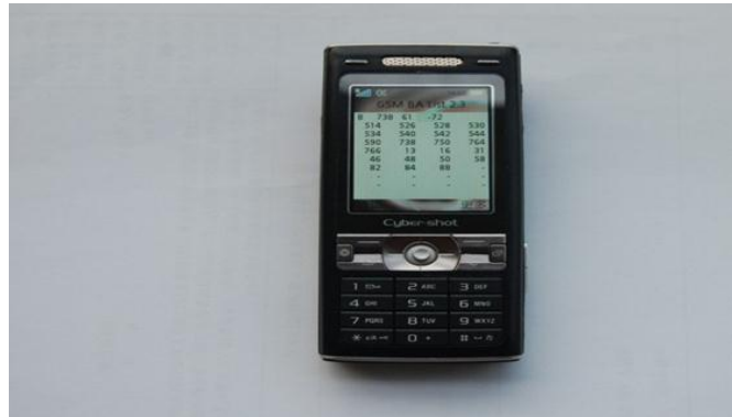
Figure-3.1. TEMS Phone for drive test
