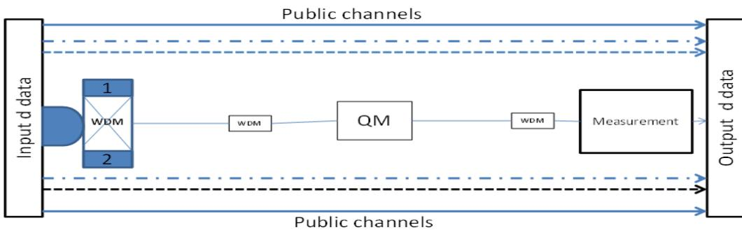
Fig-1. Schematic of network supporting QKD and WDM channels.
