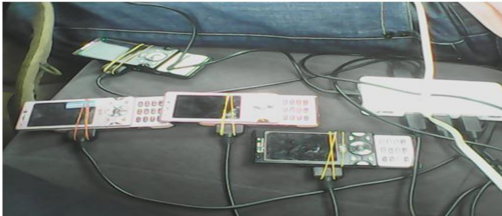
Fig-6. Drive Test TEMS Phones of the Experimental setup
