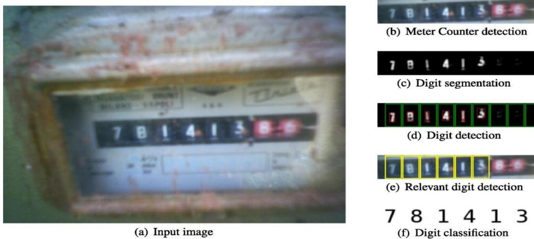
**Fig-3.** Results of the novel approach for automatic gas meter reading from the real world image
