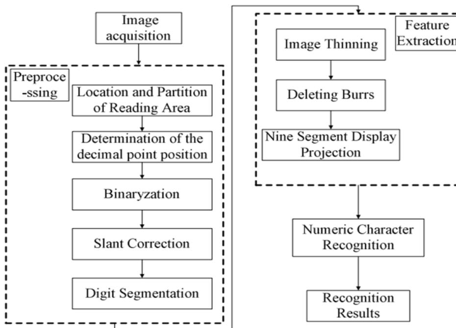
Fig-2. Flowchart of the Text Recognition in Ammeter dial Plate
