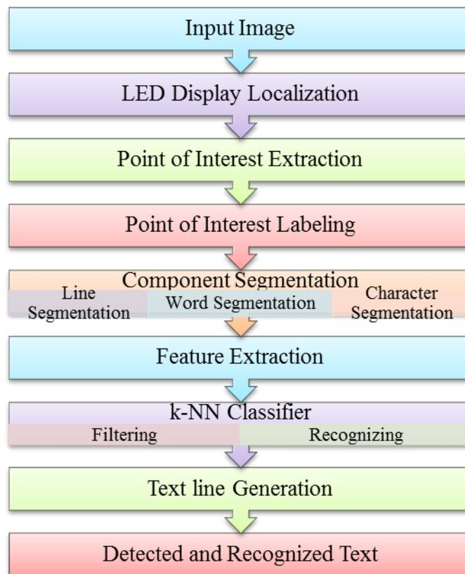
Fig-5. LED Text Detection and Recognition Process
