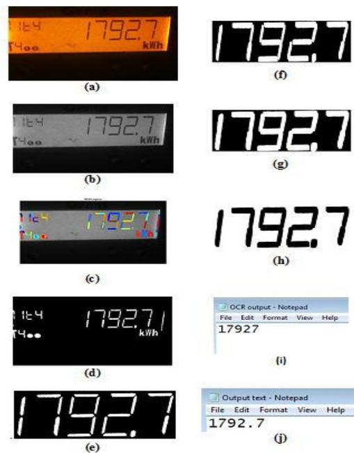
**Fig-6.** OCR Results (a) Original image sent by the consumer (b) Gray scale image (c) MSER regions (d) Binary mask (e) Cropped kWh image (f) & (g) Horizontal & Vertically dilated image (h) Complemented image (i) OCR function output (j) Final output
