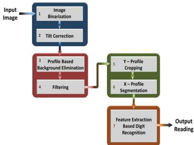
**Fig-4.** Steps Involved in the Proposed Algorithm for the Recognition of Seven Segment Numbers on Display
