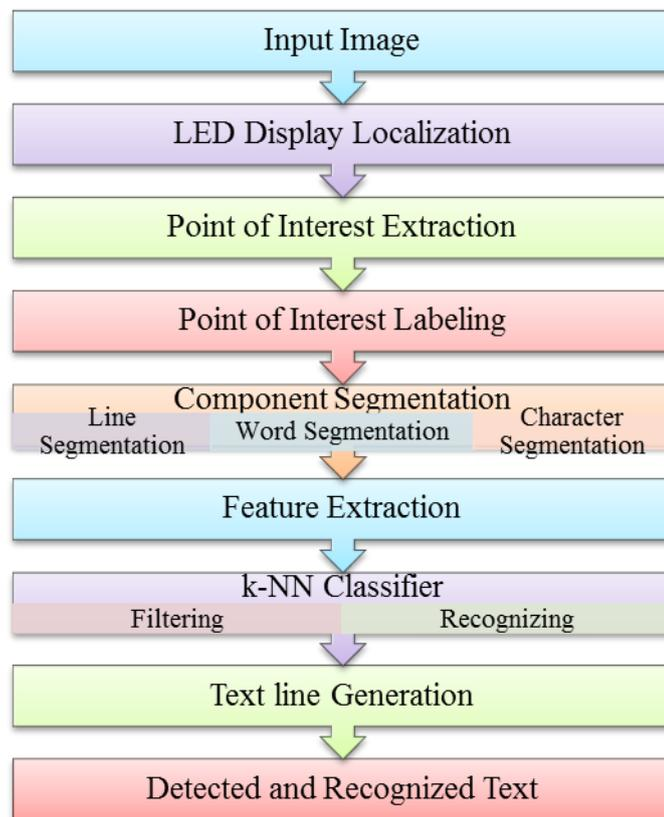
Fig-5. LED Text Detection and Recognition Process
