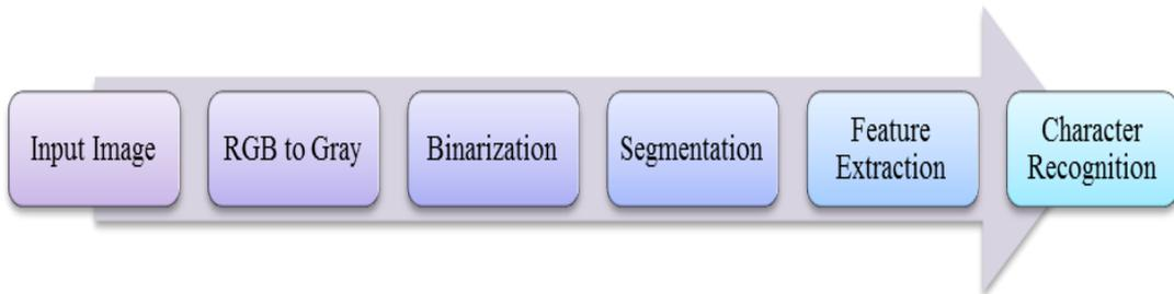
Fig-1. Various Stages Involved in Text Recognition
