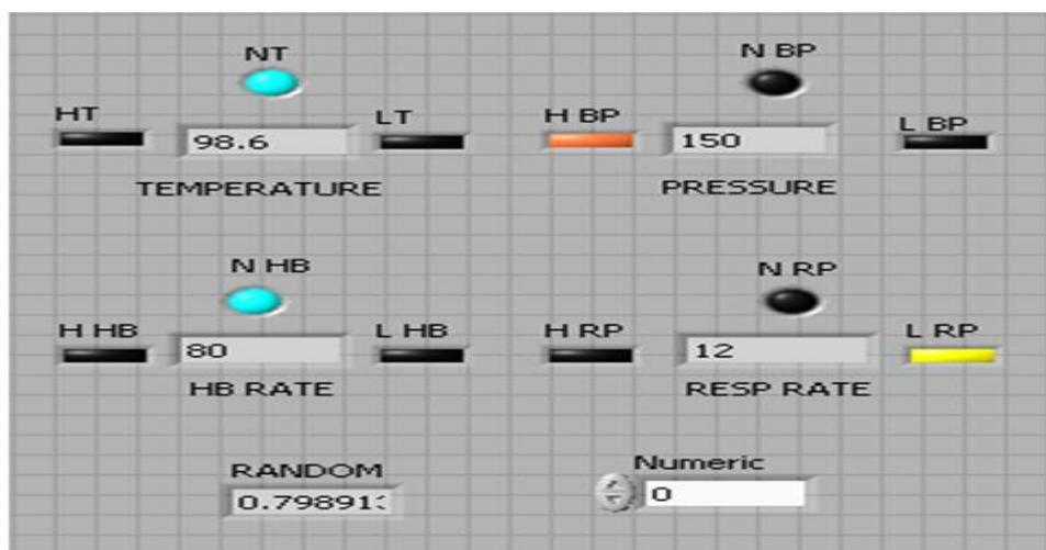
[Figure-2. Patient monitoring system -LV FRONT PANEL.](#)
