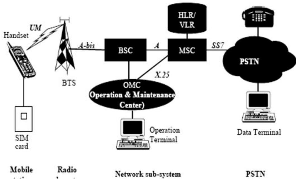
Figure-1. GSM network architecture.
