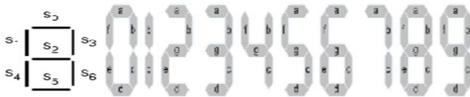
Figure-1. Seven Segment Display and Values for "0" Through "9".
