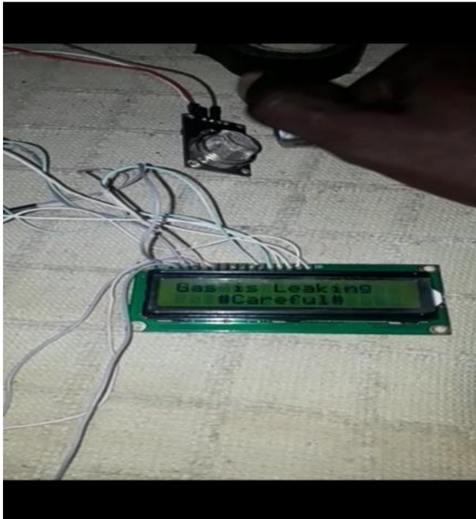
Figure-10(b). Implementation result showing gas is leaking, careful.
