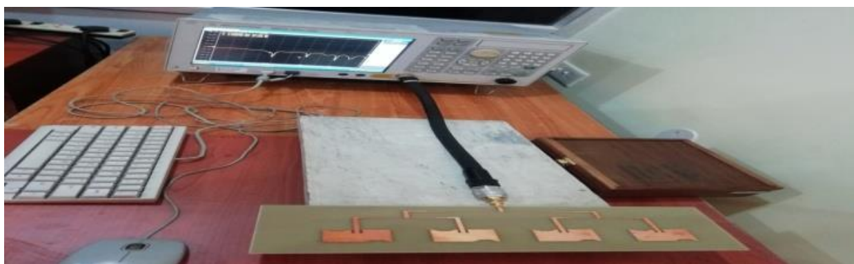
Figure 12. Measurement set up of 4 element array antenna with step cut and quarter wave transformer.
