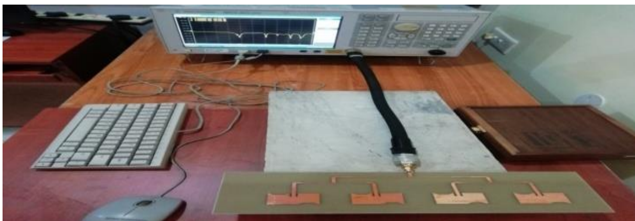
Figure 13. Measurement set up of 4 element array antenna with step cut and mitered bend feed.
