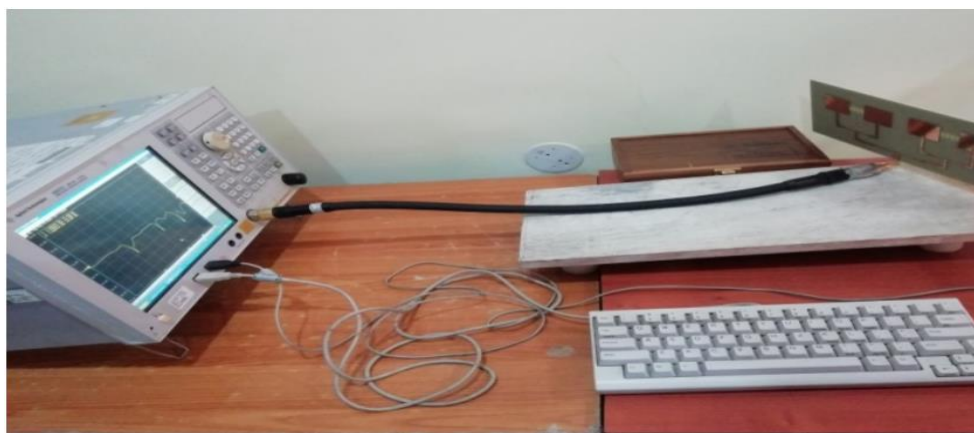
Figure 22. Measurement set up of 4 element array antenna with DGS using quarter wave transformer.
