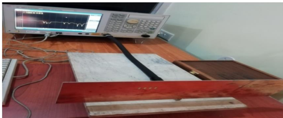
Figure 23. Measurement set up of 4 element array antenna with DGS using mitered bend feed.
