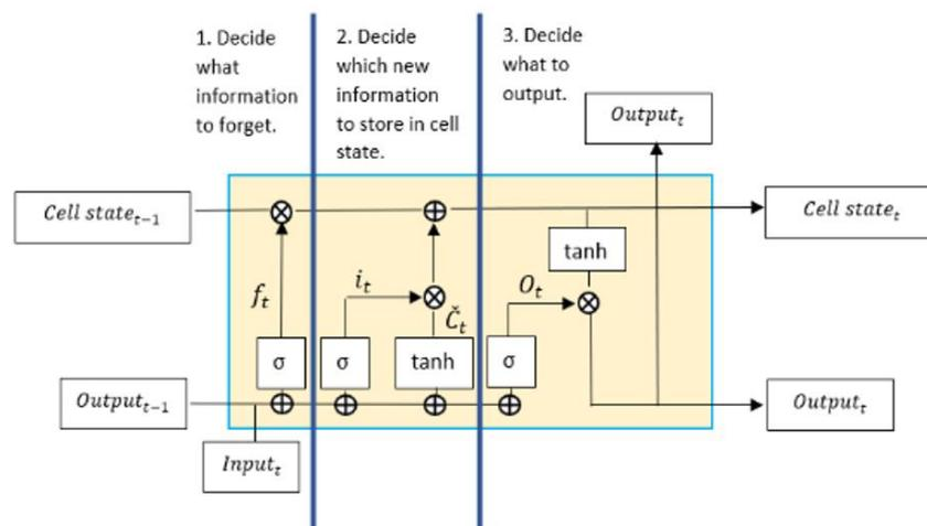
Figure 1. LSTM cell architecture and data flow.
