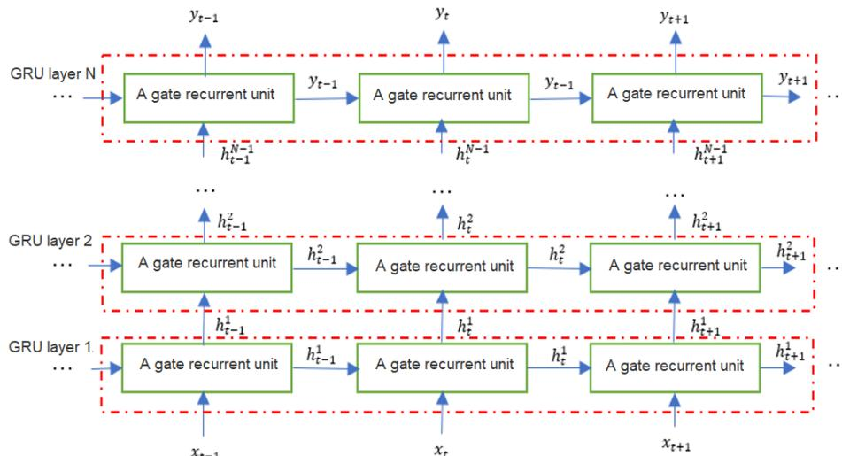
Figure 3. The architecture of a multilayer GRU.
