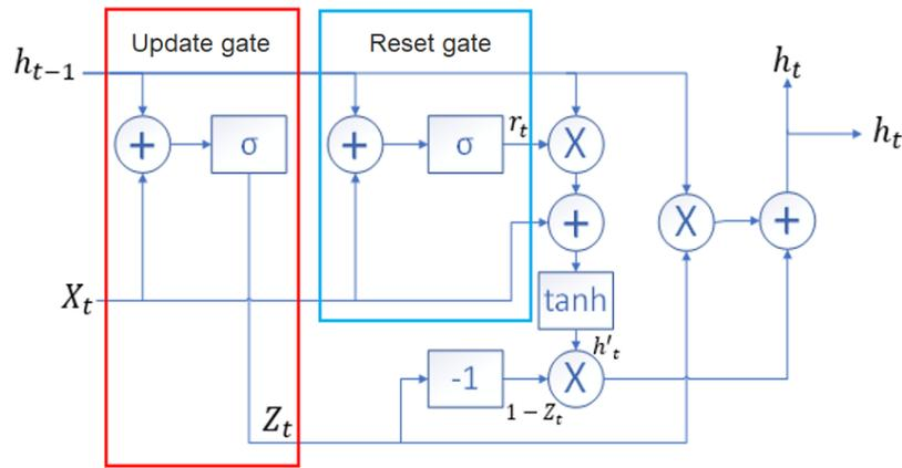
Figure 2. GRU cell architecture and dataflow.
