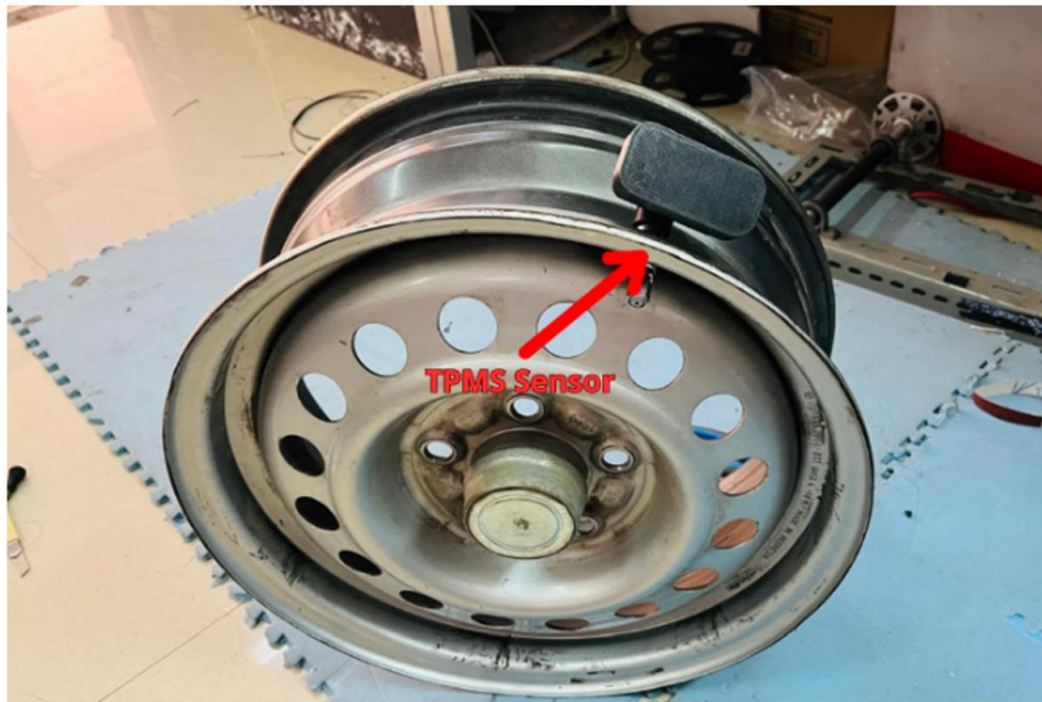
Figure 9. Installation of TPMS prototype on car alloy wheels.
