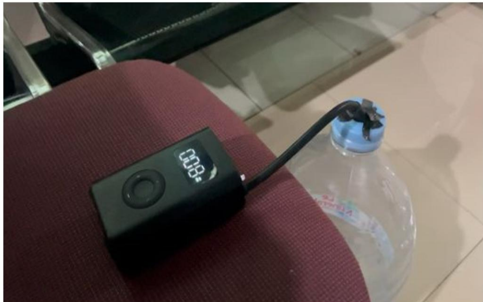
Figure 8. Pressure-filling trial with digital compressor.
