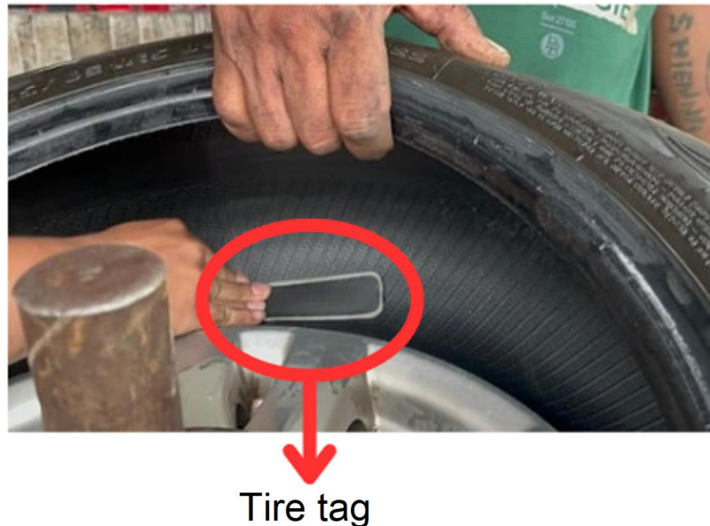
Figure 16. Installation of tire tags on vehicle tires.
