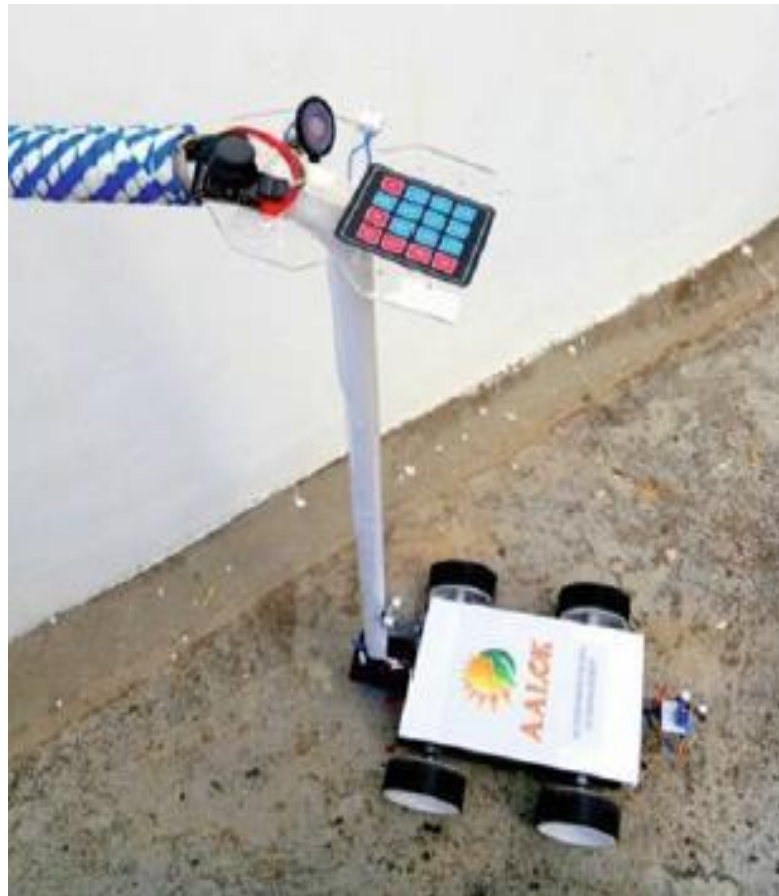
Figure 4. Design of keypad-controlled path guiding robot.
