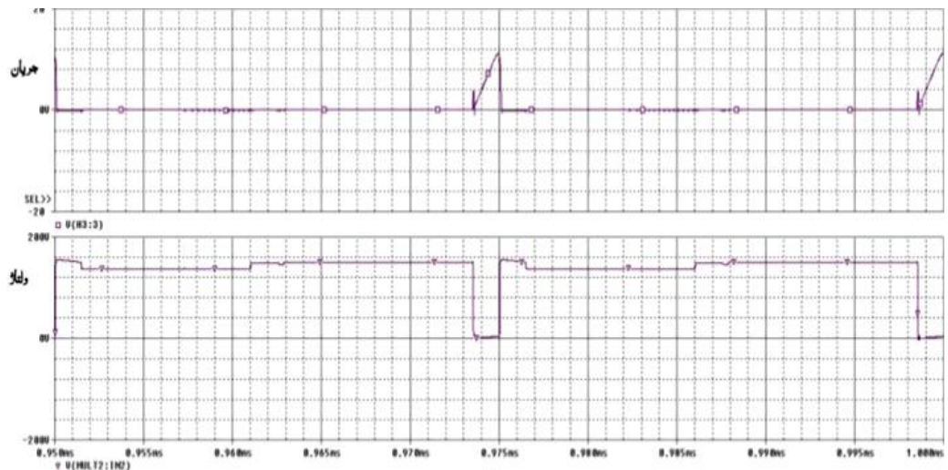
Figure-3. The shape of voltage and current waves of the secondary switch before adding Snubber
