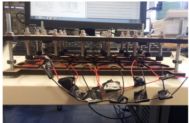
Figure-9. Prototype Harvester side-on view with piezo sensors
