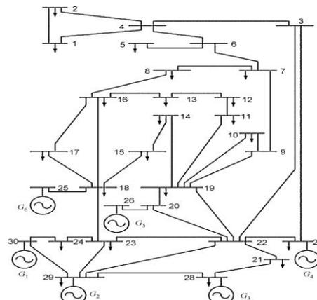
Fig-5. Single line diagram of IEEE 30 bus-6-generator test system
