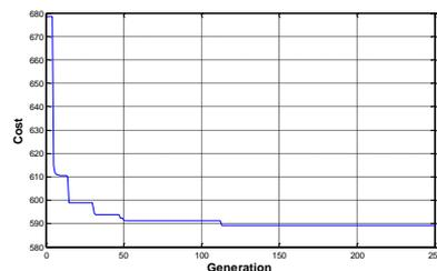
Fig-9-b. Best Cost versus generation for  $p$ -grade = 0.4
