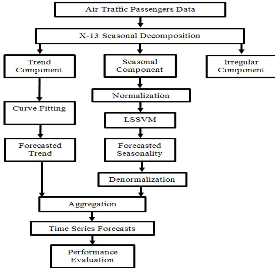
Figure-3. The process flow diagram of the proposed approach (fitted trend curve superimposed on the LSSVM seasonal forecasts).
