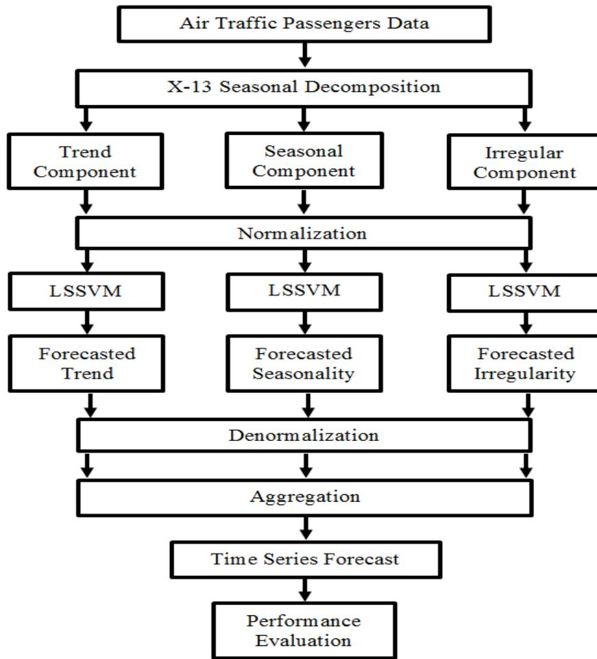
**Figure-2.** The process diagram of the hybrid X-13 LSSVM forecasting approach [14] with normalization that is not required in Xie, et al. [14].
