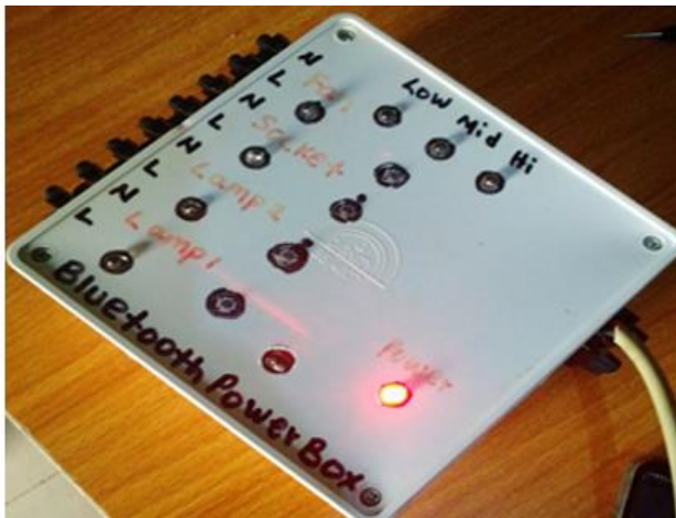
a) System ON, with all loads off
