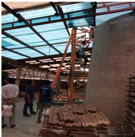
Fig-5. Measurement of CO 2 concentration in stack flue gases of brick factory using tunnel kiln technology
