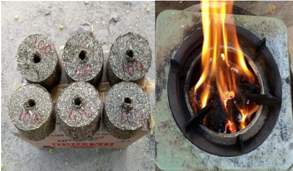
Figure-3. Sesame briquette samples and its combustion.
