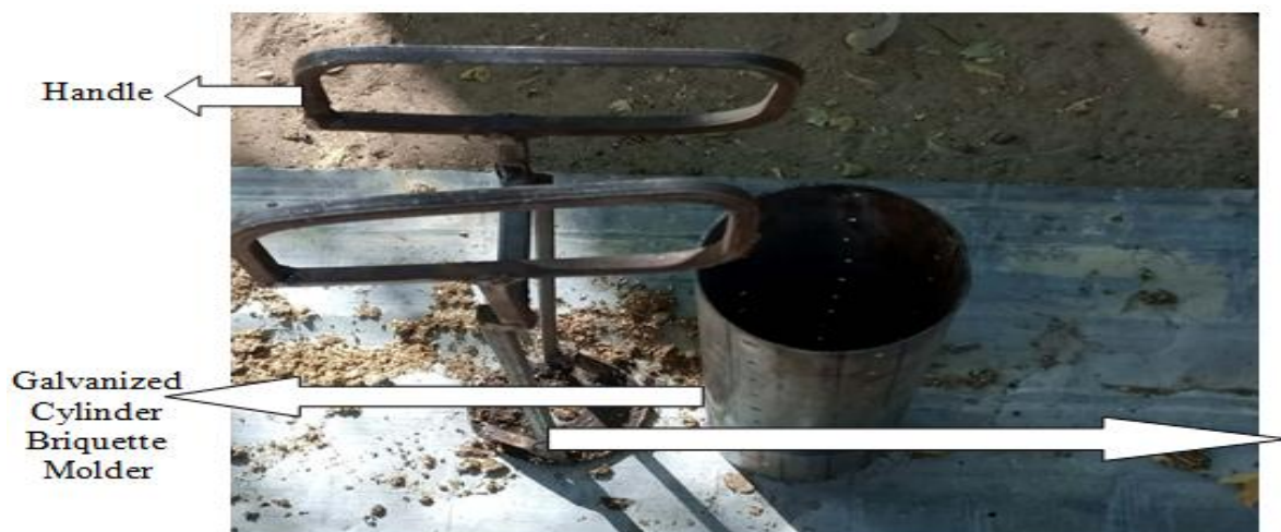
Figure-2. Fabricated manual piston briquetting machine.
