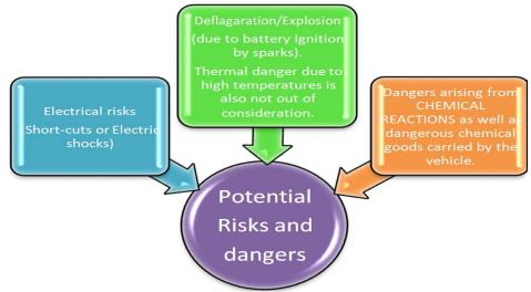
Figure-4. Potential risks and dangers of using Li-ion batteries in EVs/Hybrid vehicles.
