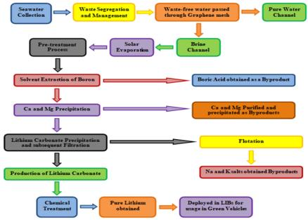
Figure-1. Flowchart demonstrating the Lithium extraction methodology.
