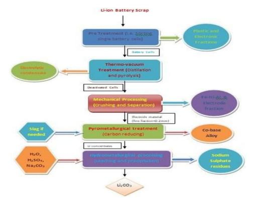
Figure-3. Flowchart showing the complete Recycling of LIB.
