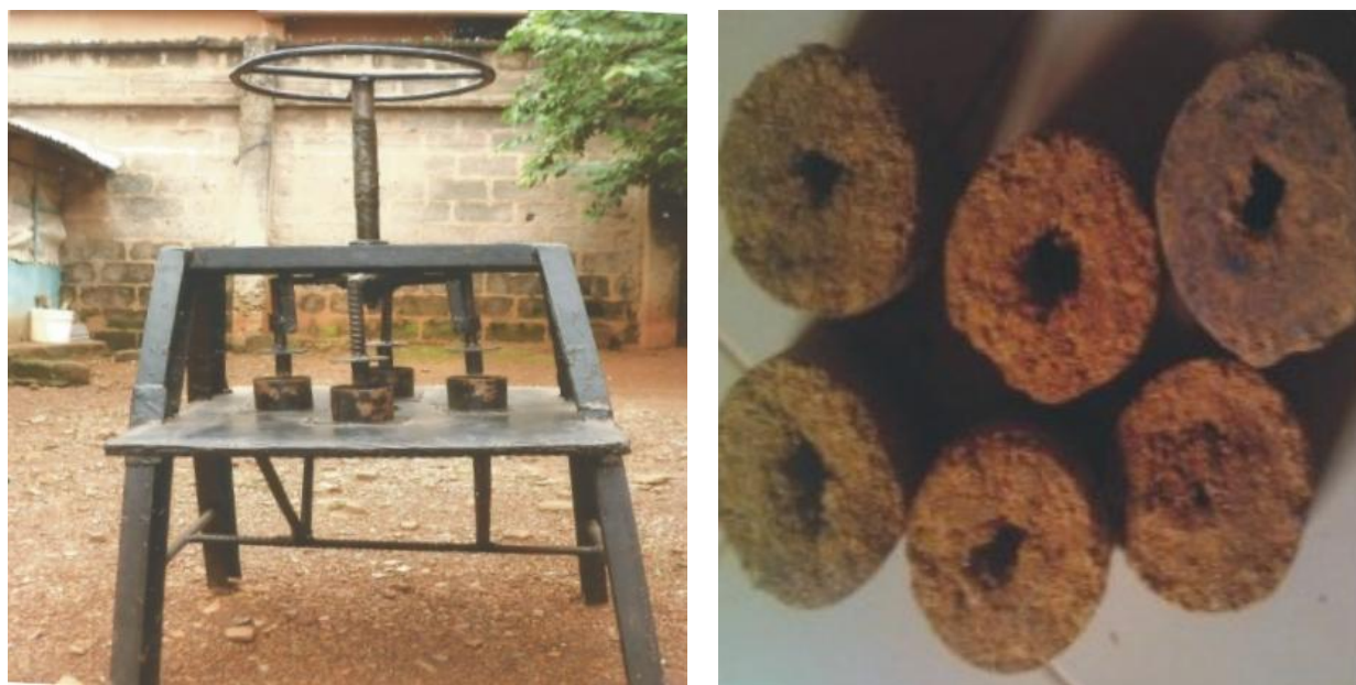
Figure-2. Manually operated screw press briquetting machine (a) and the briquettes produces (b).
