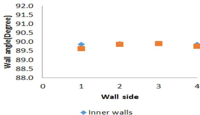
Figure-12. Position of the walls of the deposited sample after removing the base plate and re-measured 10 day after machining the surface of the sample
