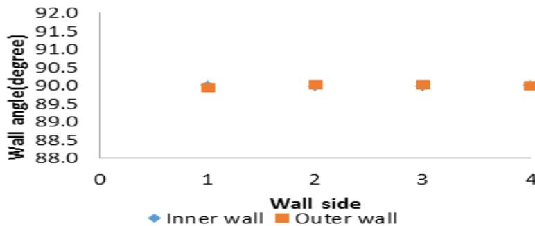
Figure-9. Position of the walls of the deposited sample before removing the base plate after machining the surface of the sample.
