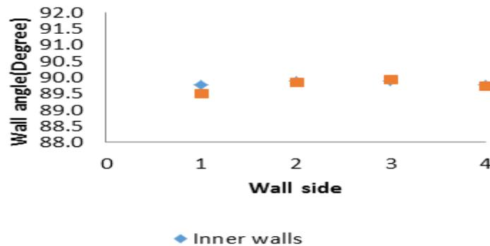
Figure-11. Position of the walls of the deposited sample after removing the base plate after machining the surface of the sample.
